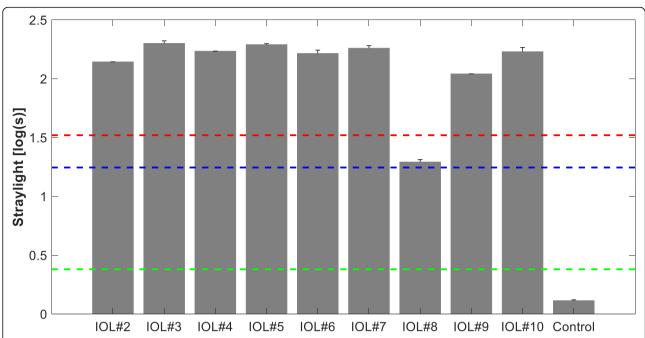
**Fig. 3** The straylight parameter of the explanted IOLs measured at a 3-mm aperture. The green and blue dashed lines are the theoretical levels of a normal 20-and 80-years-old crystalline lens. The red dashed line refers to the average straylight of an isolated cataractous lens. Error bars = standard deviation
