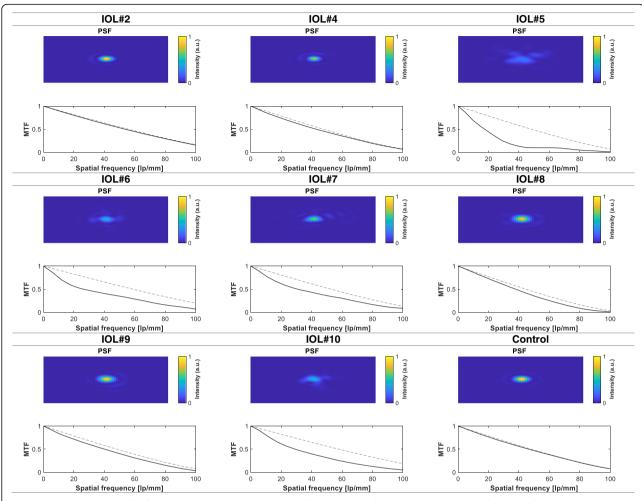
**Fig. 2** The modulation transfer function (MTF) and the point spread function (PSF) of the studied IOLs derived from wavefront aberrations at 3 mm. The dashed line is a diffraction-limited curve. Of the ten opacified lenses, measurements were possible in eight cases
