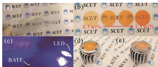
Figure 2. The (a) BATF; (b) QD films; (c) blue light spot reflection by BATFs; (d) LED assembled with a QD film; and (e) LED assembled with a BATF-QD hybrid film (5 layers of BATFs).
