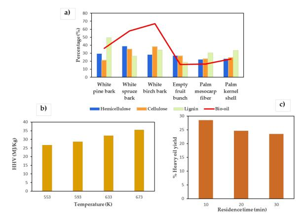
Figure 3. Effect of type of biomass (a) [99,100], temperature (b) [85,86] and residence time (c) [101] on HTL products.
