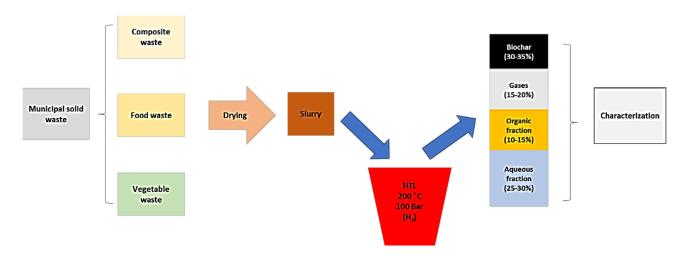
**Figure 2.** Descriptive diagram of the hydrothermal liquefaction (HTL) process from urban solid waste. Adapted from reference [90].
