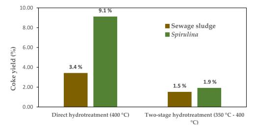
**Figure 4.** Comparison of coke yeld obtained after direct hydrotreating at 400 °C and two-stage hydrotreating. Reproduced from reference [74].
