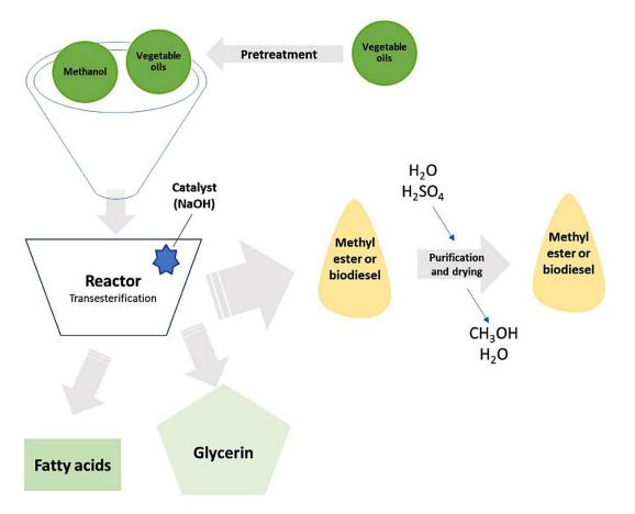
Figure 1. Biodiesel manufacturing process. Adapted from references [18,19].
