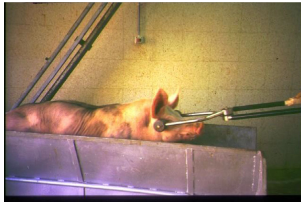
Figure 9: Head-only electrical stunning using handheld stunning tongs (source IRTA)
