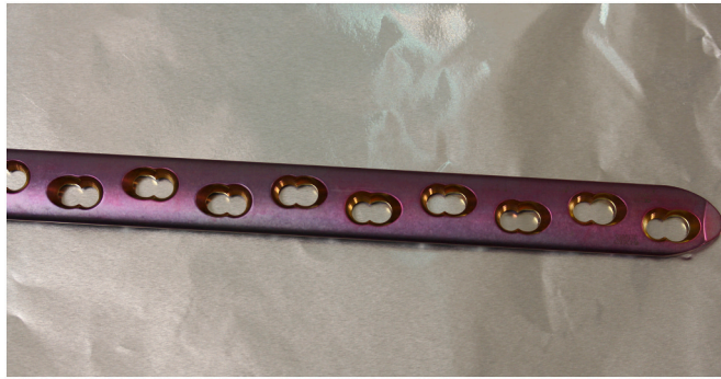
Fig. 2. Ultrathin silver plasma-coated (HyProtect®, Bio-Gate AG, Nürnberg, Germany) 12-holes LCP (DePuy Synthes®, Oberdorf, Switzerland) before implantation, which shows a slight modification of colour of the plate from gold to purple due to the plasma polymer coating process. (For interpretation of the references to colour in this figure legend, the reader is referred to the web version of this article.)
