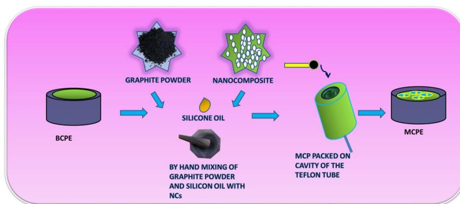
**Scheme 1.** Schematic representation of the stepwise fabrication of electrode.
