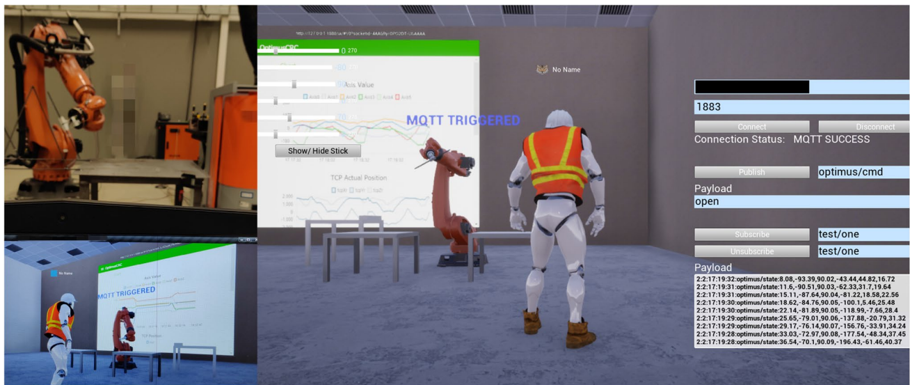
Fig. 8 Robotic DT with live-time axis value and tool position plotting
