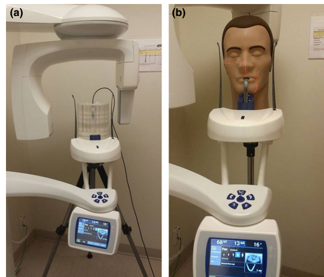
FIG. 2. Adult-sized PMMA phantom and DXTTR phantom positioned in the Planmeca ProMax 2D. (a) PMMA set-up. (b) DXTTR set-up.
