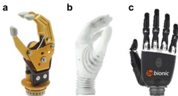
Fig. 3 Current myoelectric devices offer different options for terminal grasp, ranging from (a) two finger pinch grip to (b,c) more complex motions of the flexible wrist and finger joints (reproduced with permission of Ottobock SE & Co. KGaA.).
