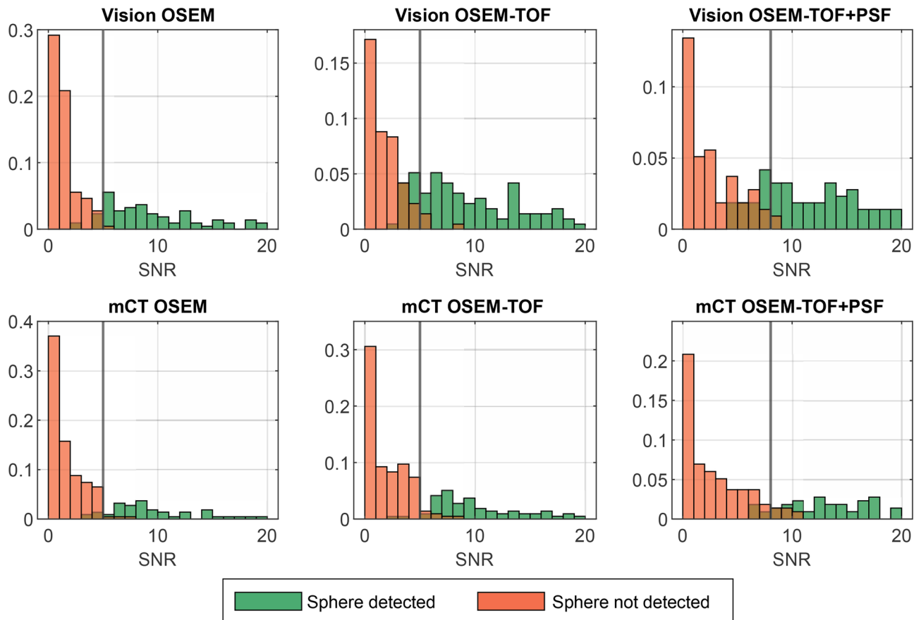
Figure 4. Normalised histograms of the SNR of detected and undetected spheres in the human observer study. Vertical lines at SNR = 5 for OSEM and OSEM-TOF image reconstruction, and SNR = 8 for OSEM-TOF+PSF image reconstruction, respectively, indicate the threshold that was derived to define a lesion as detectable in the mathematical model. For clarity purposes, SNR values > 20 are not displayed. The mixed orange-brown color arises from superposition of orange and green.
