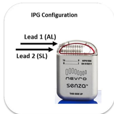
Fig. 3 Position of epidural lead (1), sham lead (2) and implantable Pulse Generator
