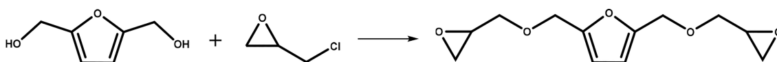
Figure 6. Reaction between BHMF and epichlorohydrin to form the diepoxy 2,5-bis[(2-oxiranylmethoxy)methyl]furan (BOF). Figure adapted from ref 66. Copyright 2012 Taylor & Francis.
