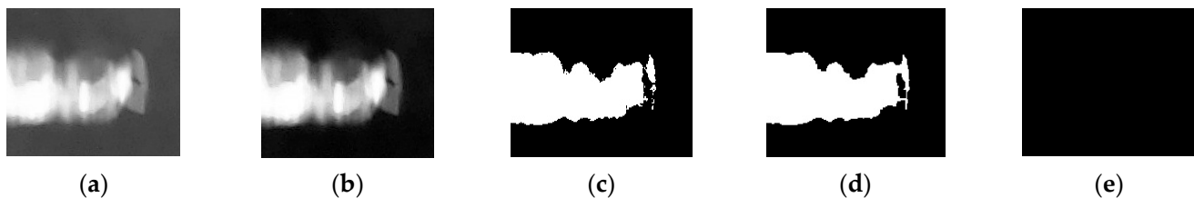
Figure 8. Processed sample of bee. (a) Original ROI; (b) Normalization; (c) Binarization; (d) Morphological processing; (e) Classification results.
