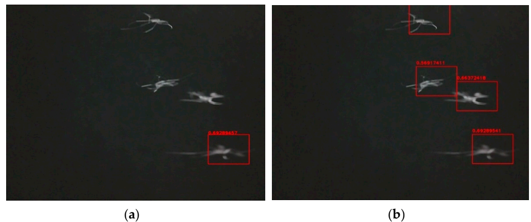
Figure 5. (a) Single template matching; (b) Multi-target template matching.
