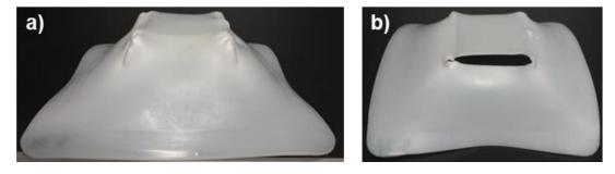
**Figure 12.** Pyramid-shaped parts made of UHMWPE (a) Sheet completely formed; (b) Sheet with failure.
