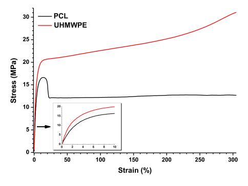
Figure 8. Tensile tests of PCL and UHMWPE.
