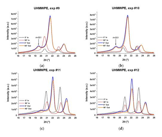
**Figure 18.** XRD patterns of UHMWPE sheets formed by SPIF through experiments (a) #9; (b) #10; (c) #11; and (d) #12. The XRD analysis was carried out separately for the inner surface (in contact with the forming tool) and the outer surface (not in contact with the forming tool) according to the experimental setup described in Figure 15.
