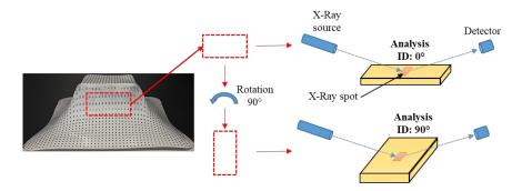
**Figure 15.** Configuration of the XRD analysis on a rectangular sample taken from the wall of the pyramid-shaped parts. The analysis were identified as " $0^{\circ}$ " and " $90^{\circ}$ " after rotation of the analyzed specimen as illustrated.
