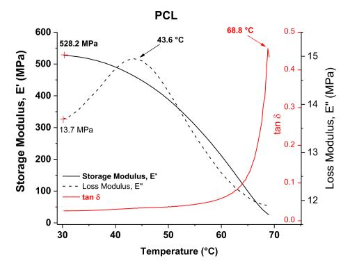
Figure 5. DMA graphs of PCL.
