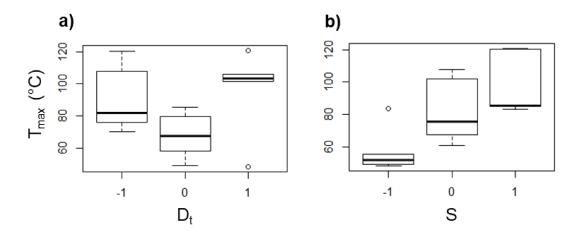
**Figure 13.** Box diagrams of  $T_{max}$  (in  ${}^{\circ}$ C) for UHMWPE as a function of (a)  $D_t$  and (b) S.
