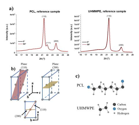
**Figure 16.** (a) XRD patterns of PCL and UHMWPE reference samples, i.e., unformed sheets; (b) Schematic representation of planes (110) and (200) of an orthorhombic crystal cell; (c) Repeat units of PCL and UHMPWE. A repetitive unit is located in each of the gray points that form the orthorhombic unit cell in (b).
