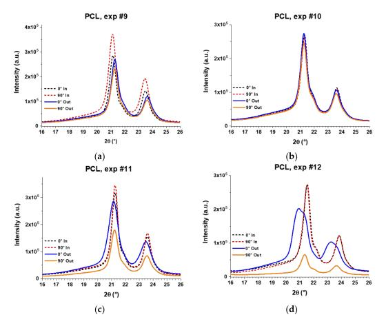
**Figure 17.** XRD patterns of PCL sheets formed by SPIF through experiments (**a**) #9; (**b**) #10; (**c**) #11; and (**d**) #12. The XRD analysis was carried out separately for the inner surface (in contact with the forming tool) and the outer surface (not in contact with the forming tool) according to the experimental setup described in Figure 15.
