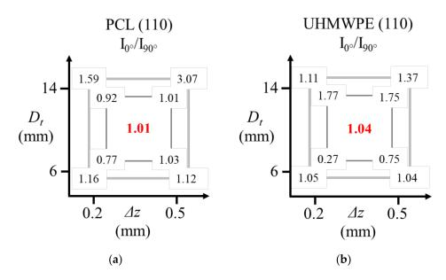
**Figure 20.** Values of the ratio  $I_0/I_{90}$  for the diffraction peak associated to the (110) plane (a) PCL; (b) UHMWPE; where  $I_0$  is the maximum intensity in the measurement at  $0^{\circ}$  and  $I_{90}$  is the maximum intensity in the measurement at  $90^{\circ}$  according to the experimental setup described in Figure 15.
