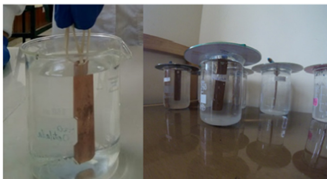
Fig. 9. Static immersion test Coupons submerged in calcium hypochlorite solution.
