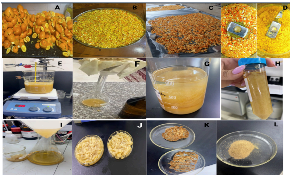
Figure 2. Process of aqueous extraction of pectin from orange peels, including washing fresh orange peels with tap water (A), cutting fresh orange peels into small pieces (B), sun-drying orange peels (C), grinding the dried orange peels (D), aqueous extraction from orange peel powder (E), filtration (F), precipitation of pectin (G), centrifugation, (H) washing pectin with HPLC-grade ethanol (I), obtaining wet pectin (J), drying the pectin (K), and pectin fine powder (L).
