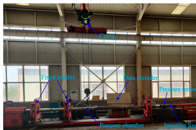
Figure 3. Pressure and temperature tests of the IPCS.
