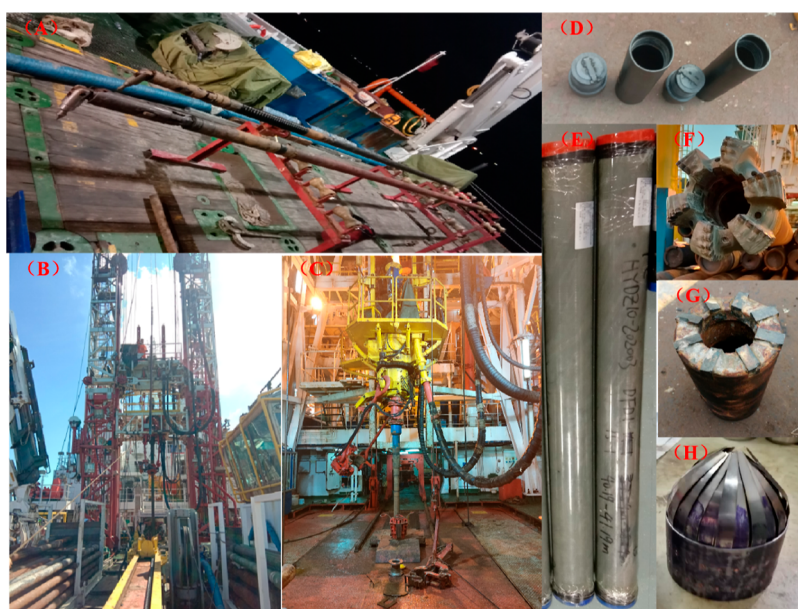
Figure 6. Offshore drilling experiments of the IPCS. (A) IPCS on the drilling vessel; (B) recovery of the CBA of the IPCS; (C) core drilling; (D) flapper valves; (E) cores from offshore drilling experiments; (F) outer core bit; (G) advanced core bit; (H) core catcher with many claws.
