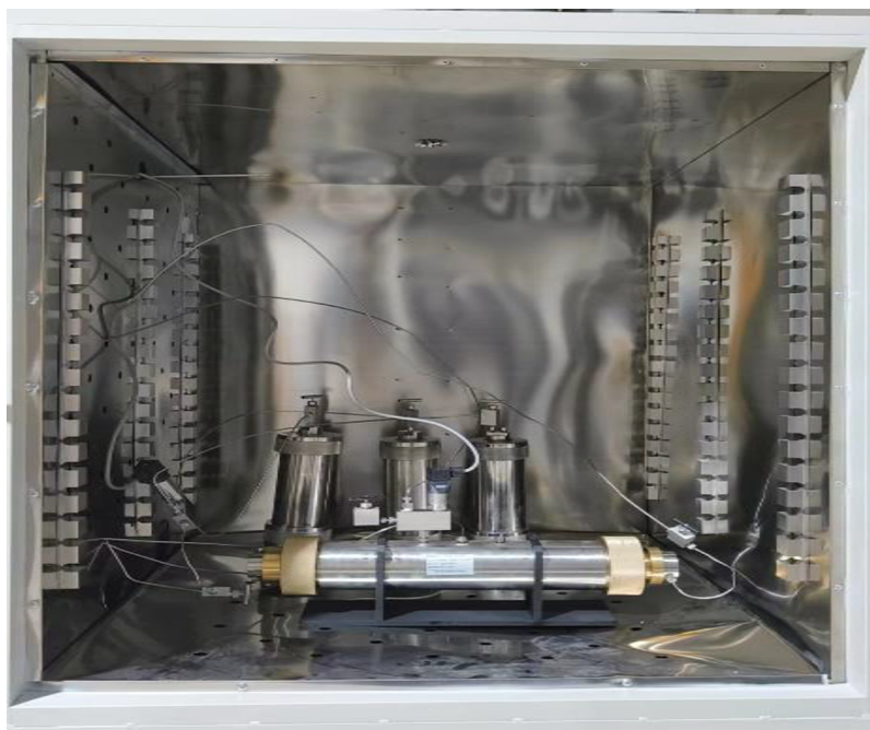
Figure 3. High-temperature and high-pressure core displacement experimental device.
