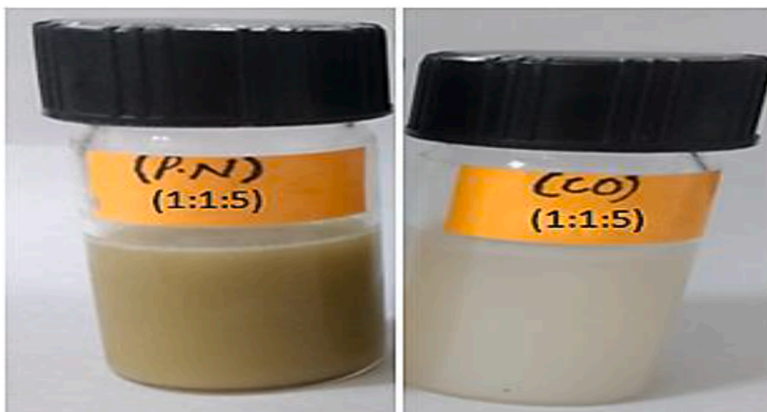
Fig. 1. Physical appearance of the prepared nanoemulsion obtained by low energy method–(PN) nanoemulsion prepared with Phyllanthus niruri extract ( P. niruri based nanoemulsion); and (CO) nanoemulsion without extract (control nanoemulsion).
