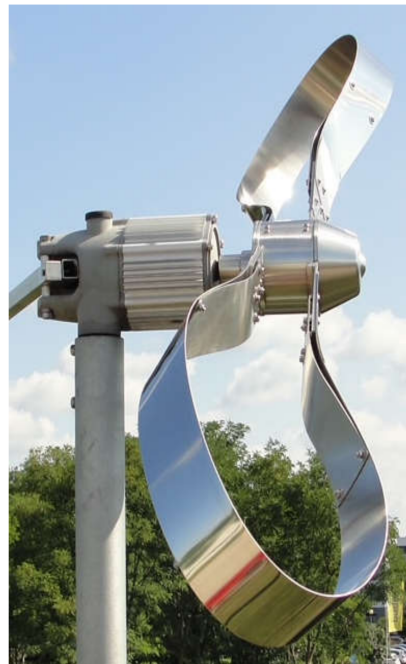
Figure 7. Wind power plant of a modernized ribbon-blade wind turbine under real conditions. Source: the authors' own materials (based on R. Kasner).
