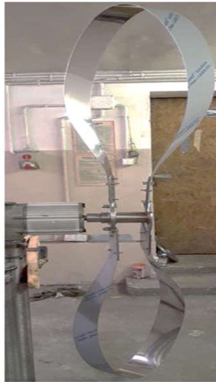
Figure 2. The manufacturing model of the rotor with ribbon blades. Source: the authors' own materials.
