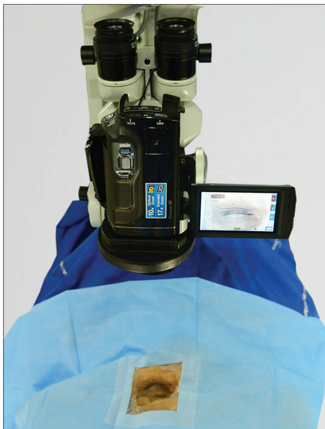
Figure 3: 4K video camera mounted paraxially on the operating microscope, showing an extended field and working distance
