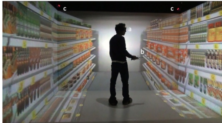
Fig. 2 Setup of the CAVE system. Experimental setup of the CAVE system: a 3D glasses; b interaction device; and c infrared tracking cameras
