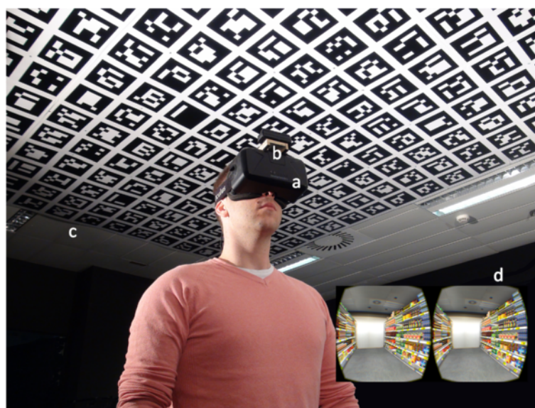
Fig. 1 Setup of the walking virtual reality system. Experimental setup of the walking virtual reality system: a head mounted display; b RGB camera; c pattern of fiducial markers; and d snapshot virtual environment that is being displayed to the user
