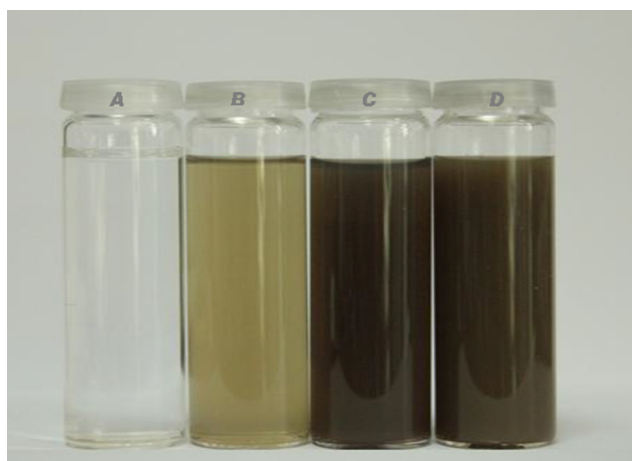
Plate 1. Tubes containing the aqueous solution of 10 -3 M of AgNO 3 with colorless at the beginning of reaction (A), after adding 1 g of P. pavonia powder with color change to yellowish brown color within 3 h (B), after adding 200 mg of P. pavonia ethanolic extract with color change to brownish black color within 2 min (C) and after adding 200 mg of P. pavonia chloroform extract with color change to dark brown color within 2 min (D).
