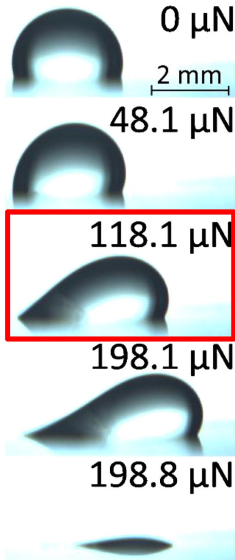
Figure 5. Pictures taken during a CAB run with 5 \mu\text{l} water drop on HeLa 64 kPa at zero normal force and growing lateral forces as noted in the figure. The image highlighted with the red box represents the moment of onset of drop detachment considered to determine the lateral retention force. The numbers on the top of the frames represent the lateral force on the drop at the time the frames were taken. Note, the onset of motion was determined from the onset of detachment of the rear end of the drop.
