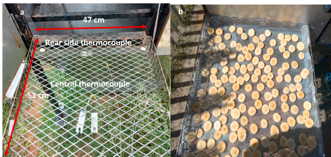
Fig. 2. (a) An empty drying tray with central and rear side thermocouples and (b) banana slices loaded on a tray with a 1 mm wire mesh placed on top of the tray during experimentation.
