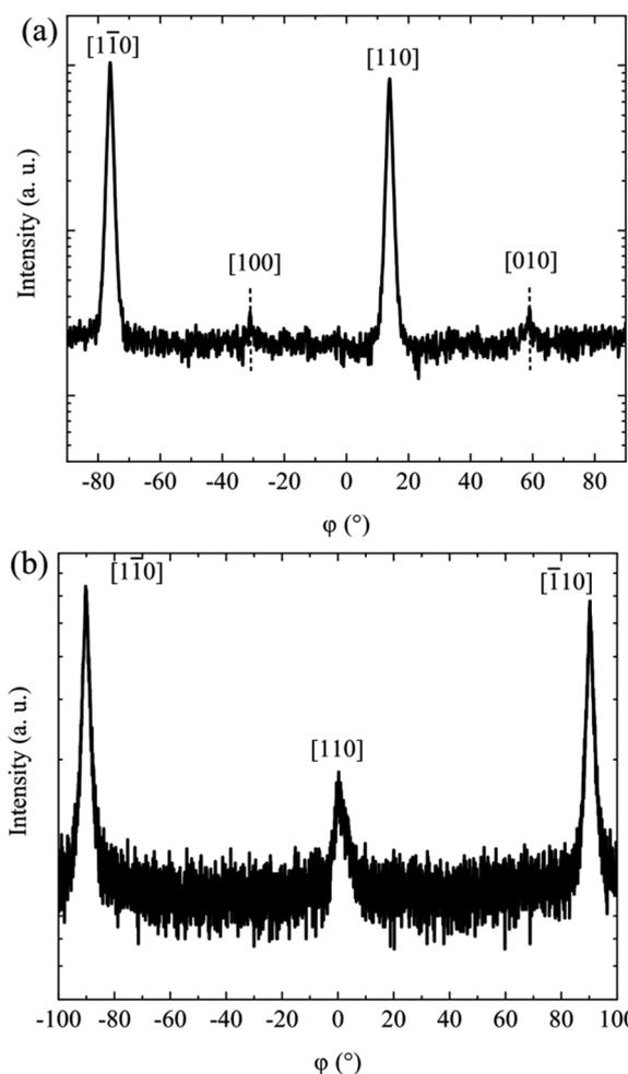
Fig. 6 (a)  $\phi$ -Scan in GIXRD geometry of the (400) reflection of the  $\text{Gd}_2\text{O}_3$  layer grown at  $p_{\text{O}_2} = 5 \cdot 10^{-7}$  mbar and (b)  $\phi$ -scan of the asymmetric 222 reflection of the  $\text{Gd}_2\text{O}_3$  layer grown at  $p_{\text{O}_2} = 5 \cdot 10^{-7}$  mbar on a  $4^\circ$  miscut substrate.
