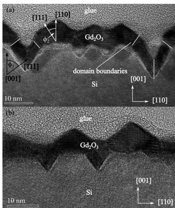
Fig. 9 TEM images of the Gd<sub>2</sub>O<sub>3</sub> layers grown at (a)  $p_{O_2} = 2 \cdot 10^{-7}$  mbar and (b)  $p_{O_2} = 5 \cdot 10^{-7}$  mbar. Some domain boundaries are marked with white lines. The angles  $\phi_1$  and  $\phi_2$  describe the angles between the orientation of the faceted silicon and Gd<sub>2</sub>O<sub>3</sub> surface, as described in the main text.
