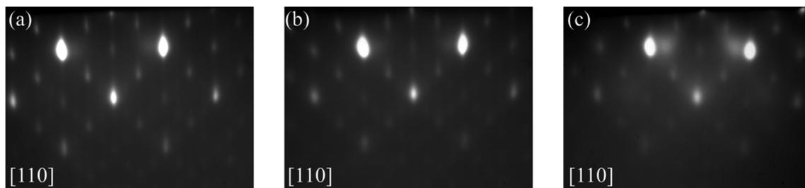
Fig. 4 RHEED images in [110] direction of the substrate of the  $\text{Gd}_2\text{O}_3$  layers after the growth at (a)  $p_{\text{O}_2} = 2 \cdot 10^{-7}$  mbar and (b)  $p_{\text{O}_2} = 5 \cdot 10^{-7}$  mbar and (c)  $p_{\text{O}_2} = 5 \cdot 10^{-7}$  mbar and  $4^\circ$  miscut Si substrates with a nominal thickness of around 10 nm.
