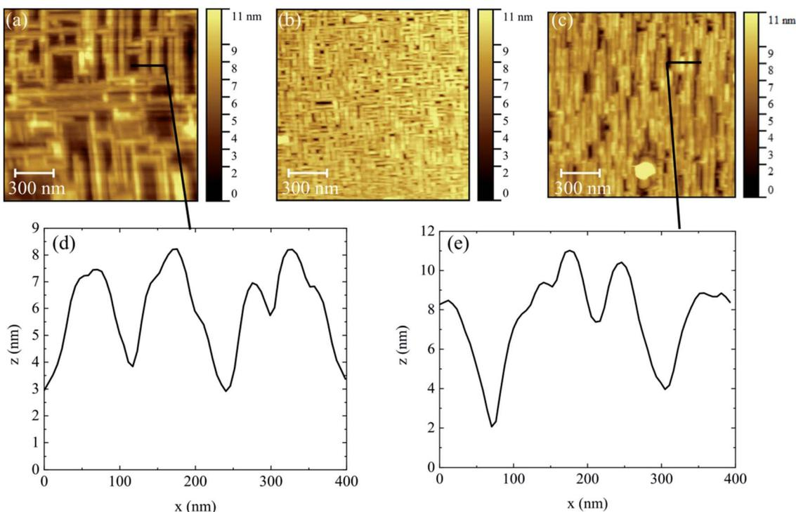
Fig. 7 AFM images of the  $\text{Gd}_2\text{O}_3$  layers grown at (a)  $p_{\text{O}_2} = 2 \cdot 10^{-7}$  mbar (b)  $p_{\text{O}_2} = 5 \cdot 10^{-7}$  mbar and (c)  $p_{\text{O}_2} = 5 \cdot 10^{-7}$  mbar on a  $4^\circ$  miscut substrate. (d) Line profile of the layers from (a) and (e) line profile of the layer from (c).
