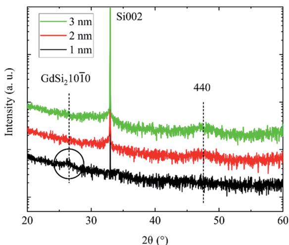
Fig. 3 Symmetric  $2\theta/\omega$  measurements of the  $\text{Gd}_2\text{O}_3$  layers grown at  $p_{\text{O}_2} = 5 \cdot 10^{-7}$  mbar with nominal thickness from 1–3 nm. The forbidden Si002 reflection is caused by "Umweganregung".<sup>47</sup>
