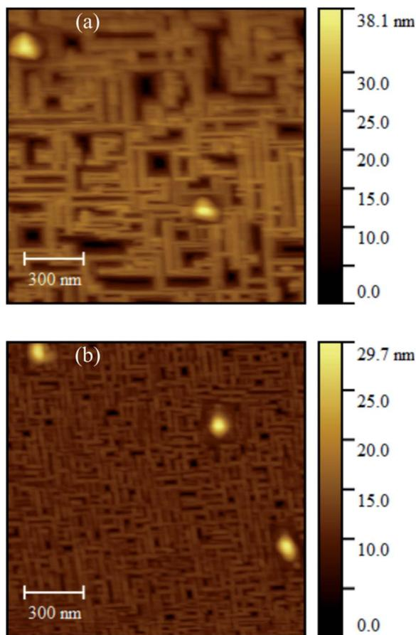
Fig. 12 (a) and (b) AFM images of  $\text{Gd}_2\text{O}_3$  layers grown at  $p_{\text{O}_2} = 5 \cdot 10^{-7}$  mbar with different nominal thickness. In both images, small islands with a height up to 20 nm can be seen.
