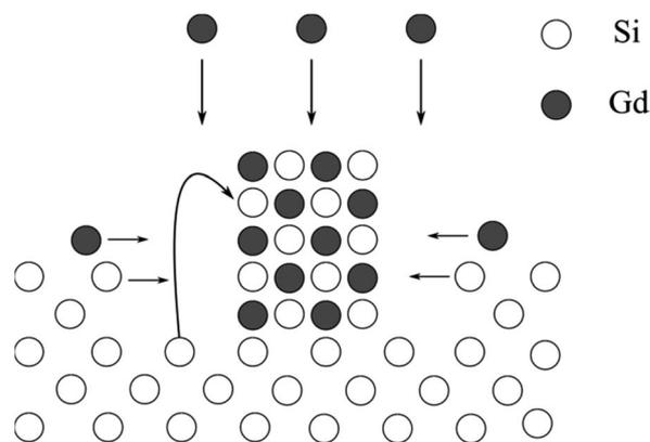
Fig. 13 Schematic drawing of the model for the formation of the silicide islands during the growth of  $\text{Gd}_2\text{O}_3$  on  $\text{Si}(001)$  at  $850^\circ\text{C}$ . The empty circles represent the silicon atoms and the filled circles represent the gadolinium atoms. Adapted from ref. 86.
