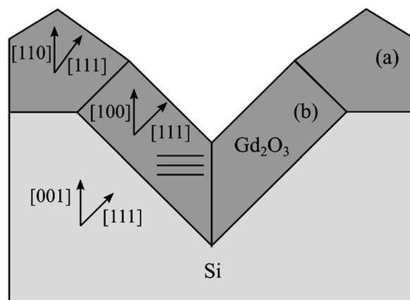
Fig. 10 Schematic drawing of the different growth regions on the faceted silicon surface. (a) Regions of Gd<sub>2</sub>O<sub>3</sub> growth on the Si(001) surface (b) regions of Gd<sub>2</sub>O<sub>3</sub> growth on {111} faceted Si surface.
