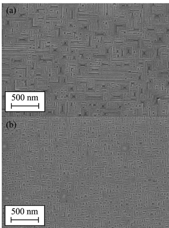
Fig. 8 SEM images of the Gd<sub>2</sub>O<sub>3</sub> grown at high temperatures and higher nominal thickness. (a) Gd<sub>2</sub>O<sub>3</sub> grown at  $p_{\text{O}_2} = 2 \cdot 10^{-7}$  mbar and (b)  $p_{\text{O}_2} = 5 \cdot 10^{-7}$  mbar.
