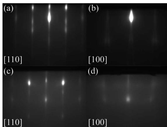
Fig. 1 RHEED images taken after the growth of the  $\text{Gd}_2\text{O}_3$  layers at  $p_{\text{O}_2} = 5 \cdot 10^{-7}$  mbar with 1 nm nominal thickness (a) in [110] direction and (b) in [100] direction of the substrate and with 3 nm nominal thickness (c) in [110] direction and (d) in [100] direction.
