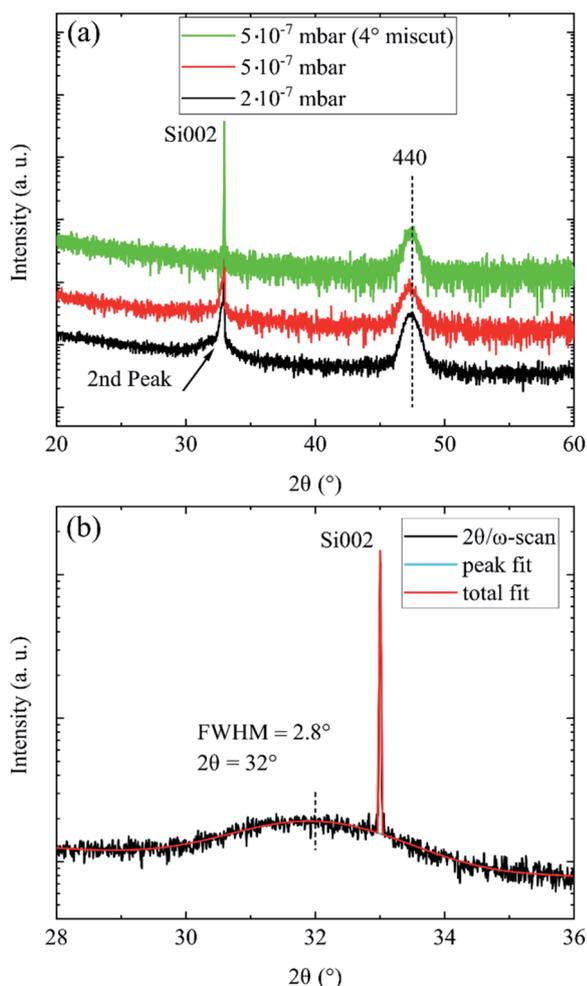
Fig. 5 (a) Symmetric  $2\theta/\omega$  measurements of the  $\text{Gd}_2\text{O}_3$  layers grown at  $p_{\text{O}_2} = 2 \cdot 10^{-7}$  mbar,  $p_{\text{O}_2} = 5 \cdot 10^{-7}$  mbar and  $p_{\text{O}_2} = 5 \cdot 10^{-7}$  mbar and  $4^\circ$  miscut Si substrates with a nominal thickness of around 10 nm. (b) Symmetric  $2\theta/\omega$  measurements of the  $\text{Gd}_2\text{O}_3$  layers grown at  $p_{\text{O}_2} = 2 \cdot 10^{-7}$  mbar with a higher signal to noise ratio.
