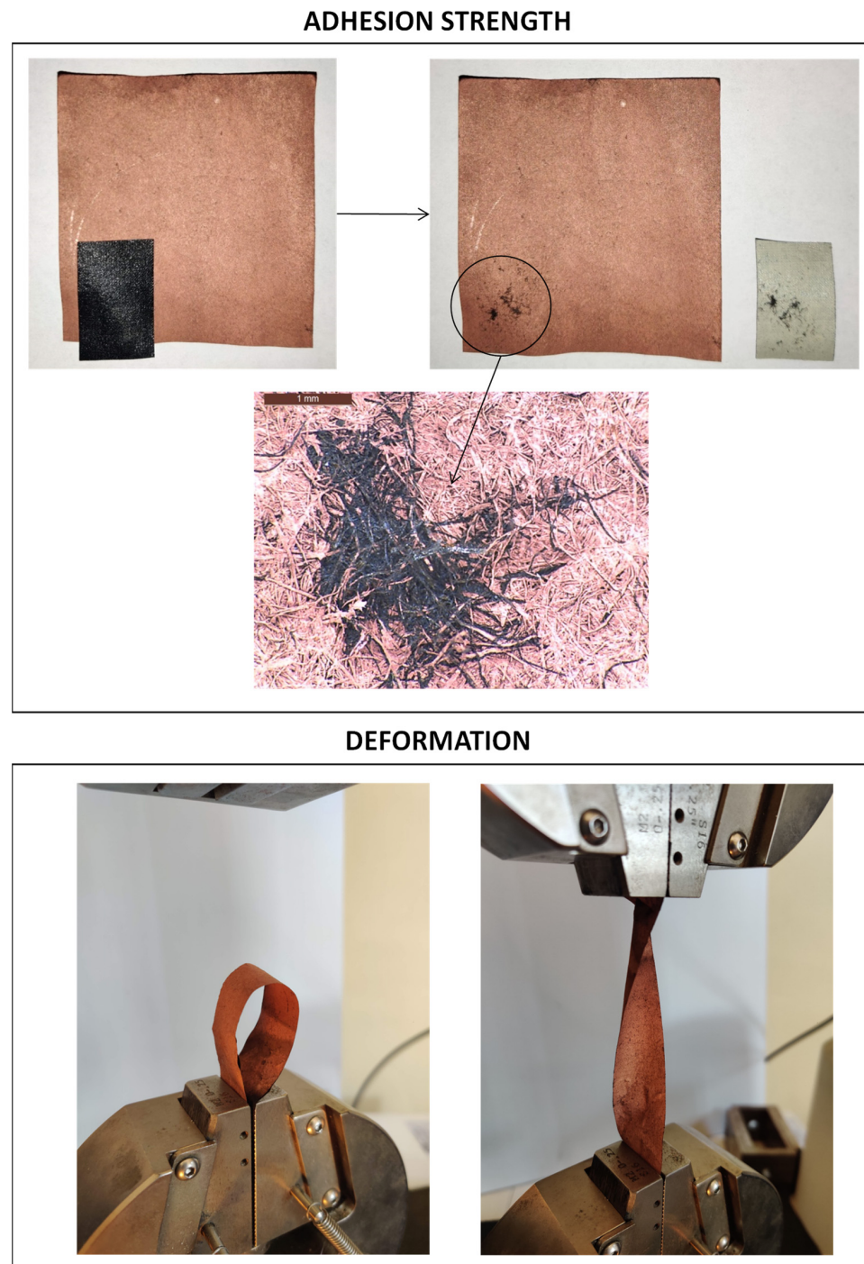
Figure 8. Adhesive strength and susceptibility to deformation of the deposited copper layer.
