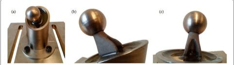
**Fig. 5** Experimentally tested prototype. (a) Prosthesis embedded in resin. (b) Detailed view of the undamaged neck of the prosthesis after experimental testing. (c) Detailed view of the undamaged neck of the prosthesis after experimental testing from a different perspective
