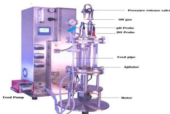
Fig. 1. Laboratory scale bioreactor.
