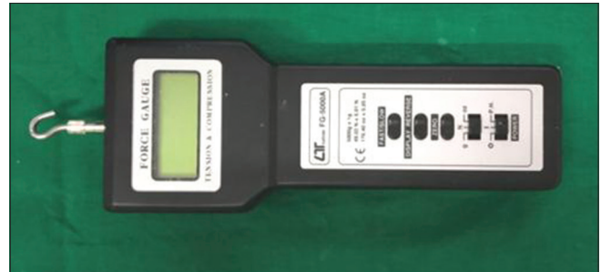
Figure 5: Digital force gauge with the hook (FG 5000A, Lutron Electronic Enterprise Co., Ltd. Taipei)
