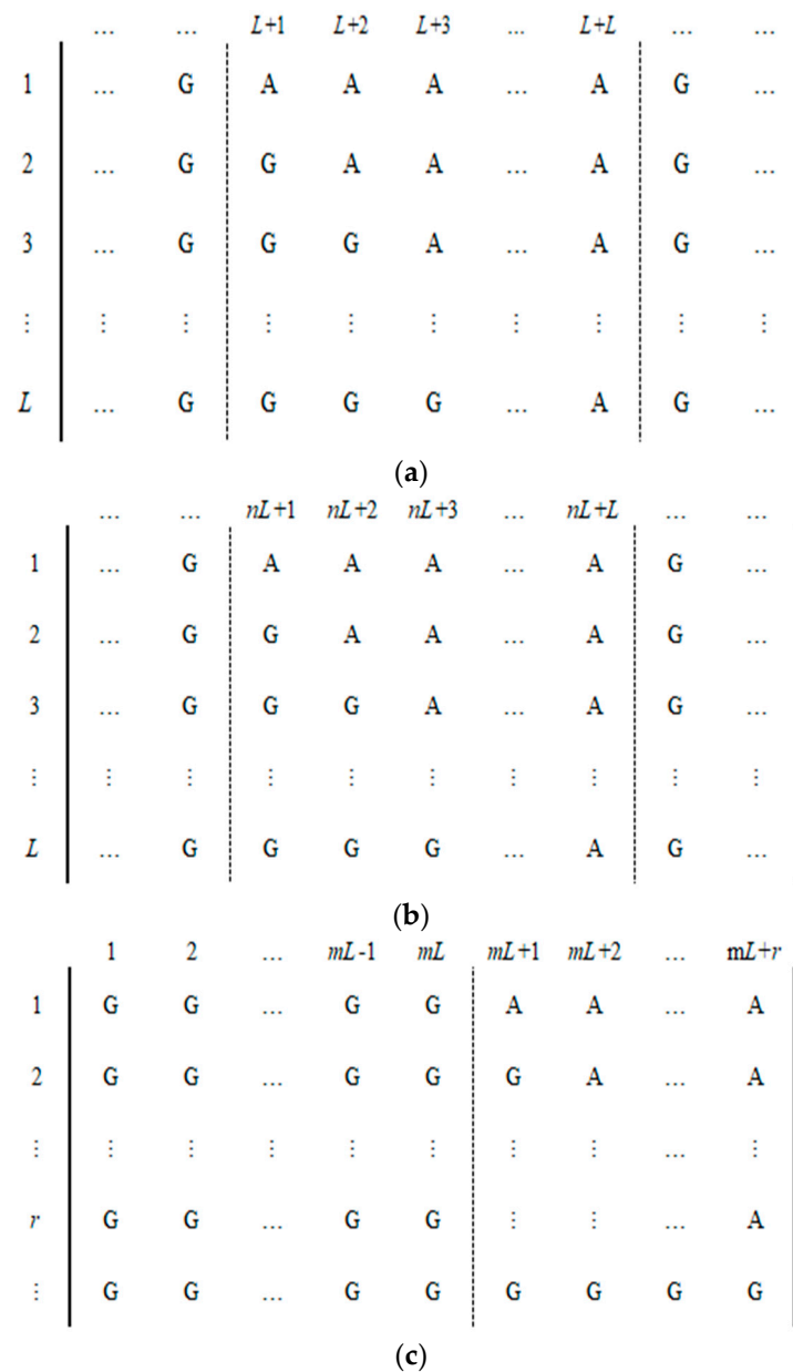
Figure 3. The encoded images of m chosen-plaintext images for the case M < 4N . (a) The first encoded image. (b) The n -th encoded image. (c) The last encoded image ( 0 \leq r < L ).
