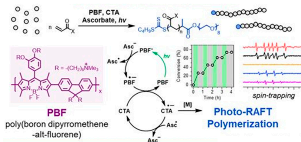
Figure 11. Photo-controlled RAFT polymerization of acrylic monomers, using the conjugated polymer PBF as the photocatalyst [80].
