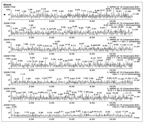
Figure 1: Mass chromatogram of blank solid matrix – Psyllium husk; No peaks of glibenclamide, glimepiride, glipizide, rosiglitazone, gliclazide, clomipramine (IS) and metformin
