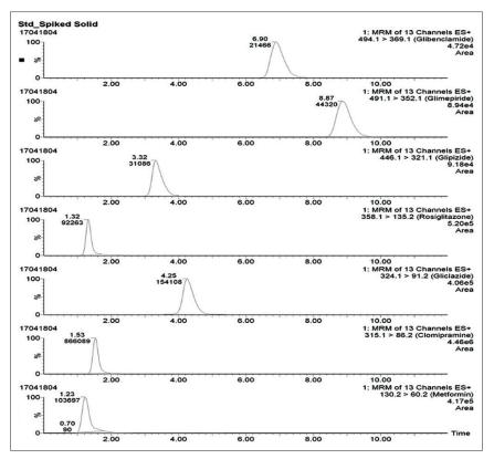
Figure 4: Mass chromatogram of the spiked solid matrix: Retention time and abundance of glibenclamide, glimepiride, glipizide, rosiglitazone, gliclazide, clomipramine (IS), and metformin
