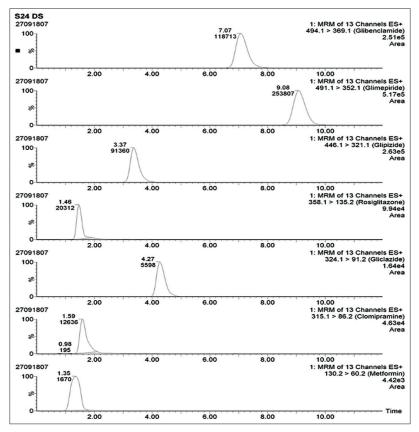
Figure 8: Mass chromatogram of intentionally spiked solid HM sample number 24 shows peaks of all antidiabetic analytes
