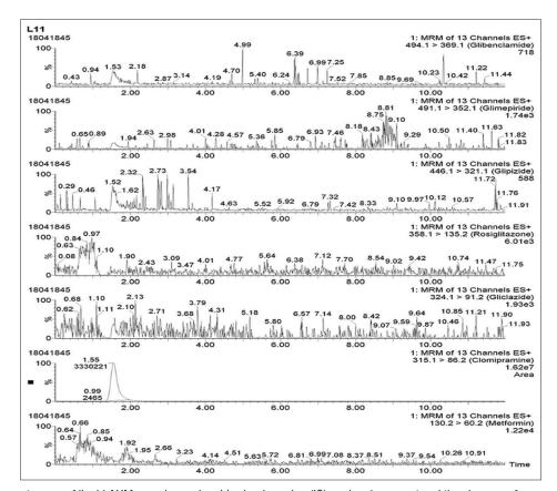
Figure 7: Mass chromatogram of liquid AHM sample number 11. clomipramine (IS) peak only present and the absence of proposed adulterants peak
