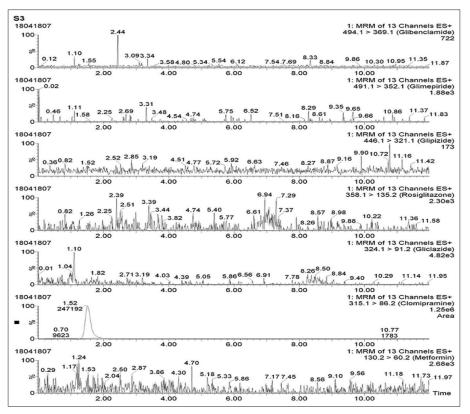
Figure 6: Mass chromatogram of solid HM sample number 3: Presence of clomipramine (IS) peak only and the absence of proposed adulterants peaks
