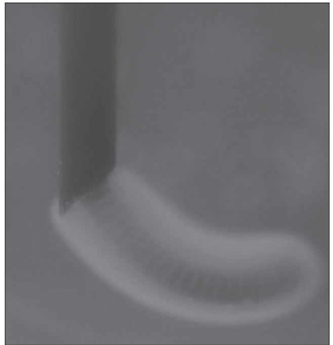
Figure 2) Photograph of a lesion generated in egg white using the Tew electrode (Tew-CTC, Radionics, USA) at 75°C for 30 s
