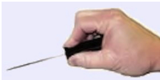
Fig. 5. Illustration of the pinch grip: The tool is gripped between the thumb and the fingertips.
