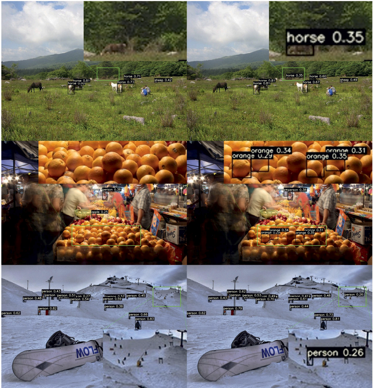
Fig. 6. Visual performance comparison. Left: YOLOv7-W6. Right: ASSN + YOLOv7-W6. Only detection results for small objects smaller than 32×32 were visualized. It can be seen that ASSN is detecting more small objects in the area of green rectangles in each figure.
