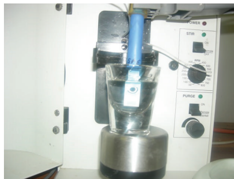
FIGURE 1: The electrochemical cell: (a) screen printed carbon electrode, counter carbon electrode, and Ag reference electrode; (b) connector cable with the electrochemical cell.
