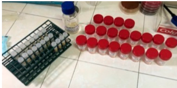
Figure 2. Containers with prepared teeth and metal brackets attached to them, before performing the bacterial inoculation with a 0.2 mL suspension of Streptococcus mutans .
