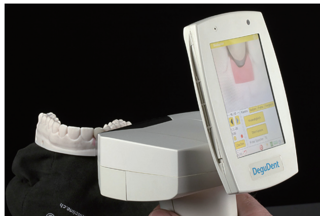
Fig. 5. In vitro color measurement using the spectrophotometer.
