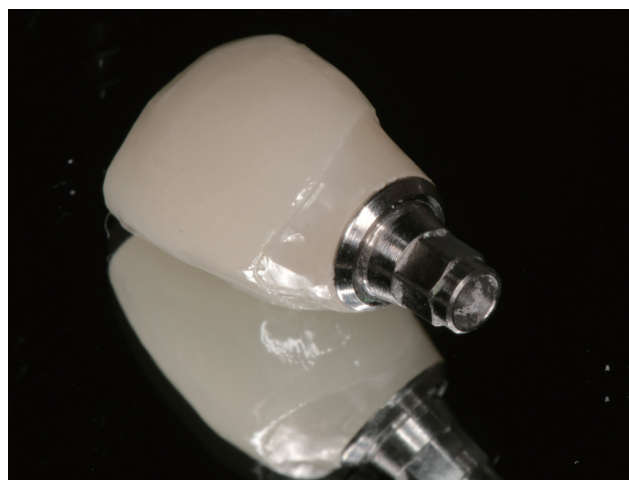
Fig. 3. Ti-base hybrid specimen with cemented all-ceramic crown.
