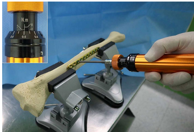
Figure 1. To overtighten and jam the locking screws into the locking plates by applying an identical torque, a torque driver with the torque limit set at 4.5 Nm was used (upper left box). A total of 120 screws were overtightened by applying an identical torque of 4.5 Nm, which exceeded the recommended torque of 1.5 Nm for the 3.5-mm locking screw insertion.
