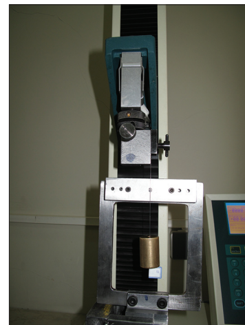
Figure 3: Friction measurements by means of a universal testing machine
