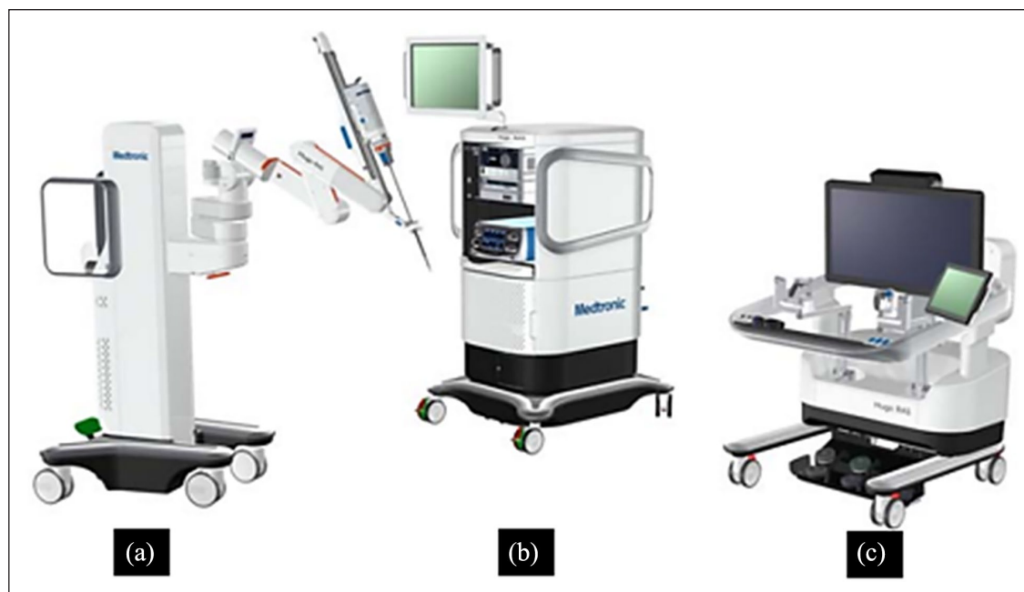
Figure 1. Components of the Hugo™ RAS system: (a) arm carts, (b) system tower, and (c) surgeon console.
