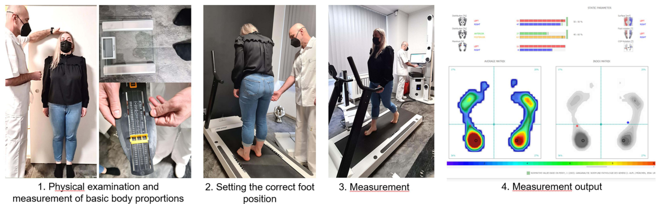
Figure 1 Methodical diagram of the measurement procedure with Diers 4D Motion Lab. Subjects provided consent for a published photo.
