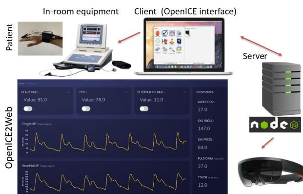
**FIGURE 5.** Architecture of Holoknee intraoperative support for monitoring and visualization of patient vital signs. Interoperability was ensured by OpenICE protocol. The present test reports blood pressure, heart rate, and SpO2 recorded by the medical-certified Finometer system.
