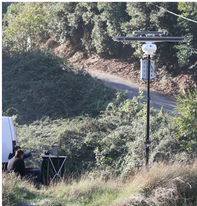
Figure 1. Standard radar setup operating in a hilly and woody environment. The TX and RX antennas are visible on top of the system, while the 4U case rack is hanging right below the rotary joint. A telescopic tower helps to lift the radar up to about 6 metres to avoid obstacles.
