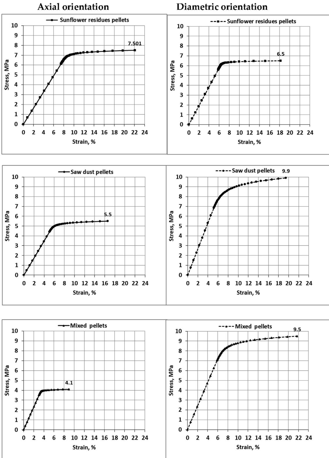
Fig. 2. The relationship between compressive stress and strain for different biomass pellets at axial and diametric orientations.
