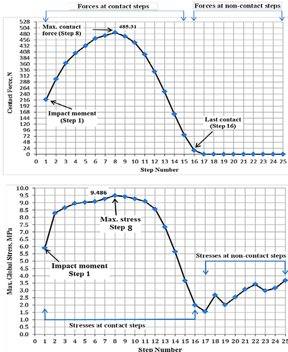
Fig. 3. Contact force and maximum stress of the mixed pellet under drop steps.
