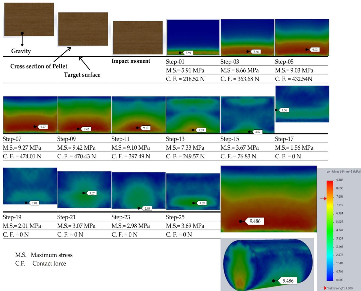
Fig. 4. A dropping test for a modelled mixed pellet in (0°) horizontal orientation dropped from 20000 mm on rigid target.
