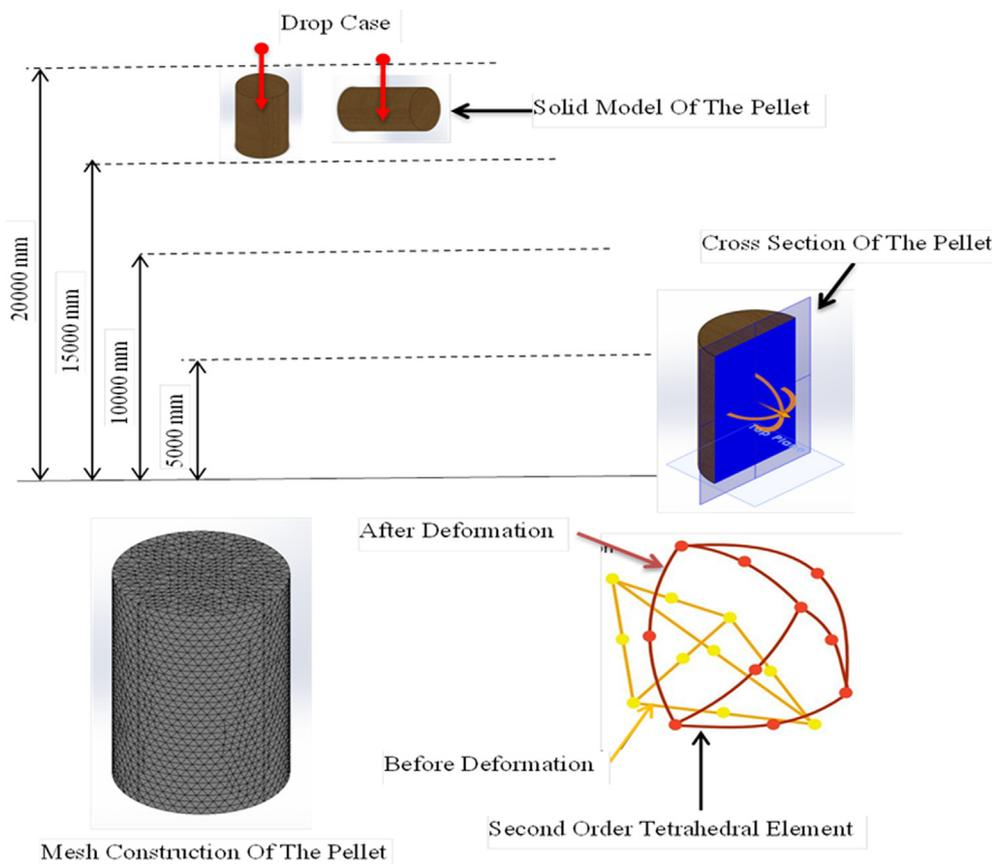
Fig. 1. 3D solid modelling, mesh construction and drop cases of biomass pellet.
