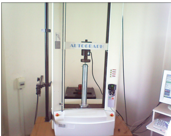
Figure 2: Application of the test on the axial compression testing machine
