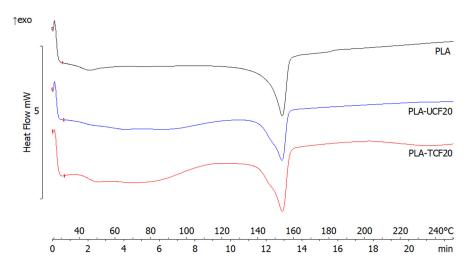
Figure 8. DSC curves of films with and without CF treatment.
