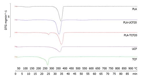
Figure 7. DTG curves of films and fibers with and without treatment.
