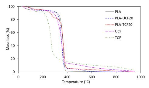
Figure 6. TGA curves of films and fibers with and without treatment.
