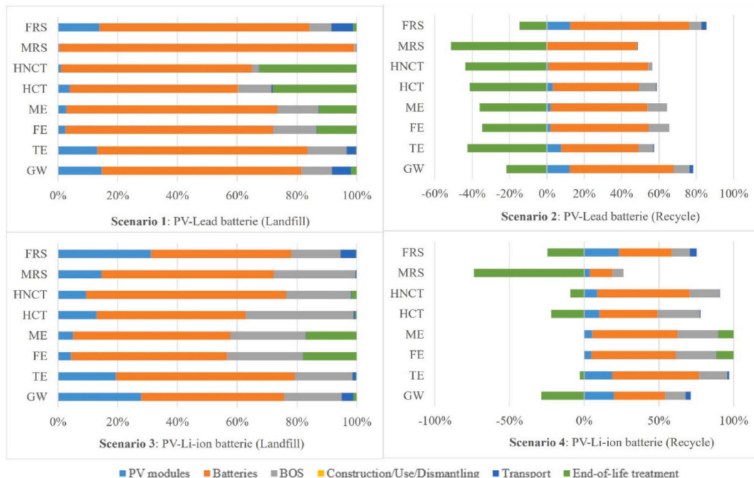
Fig. 3. Results of the characterization of the electricity production by the 04 scenarios studied.
