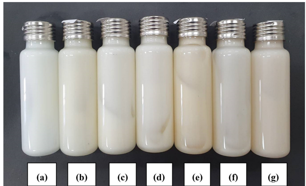
Figure 4. Deodorant cream with 1.5% H-CMCH by heating/cooling cycle; (a) cycle 0, (b) cycle 1, (c) cycle 2, (d) cycle 3, (e) cycle 4, (f) cycle 5, and (g) cycle 6.
